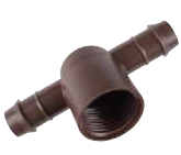
PLD-075-TBT-EE T 17 mm portagomma x 3/4" (19 mm) filettato femmina
